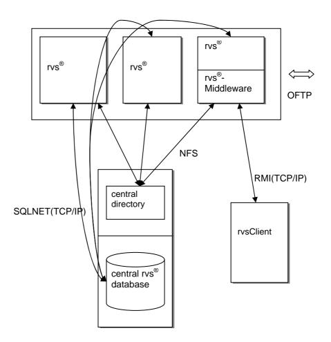
Connecting networks (ISDN, X.25 or TCP/IP) for file transmission or reception must be set up on all rvs<sup>®</sup> nodes. The above illustration shows this component with OFTP.
